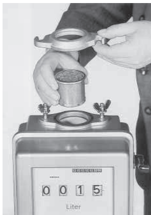
Quantity preset register with desiccant cartridge removed
